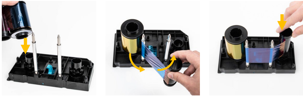
Figure 13 Loading the ribbon
