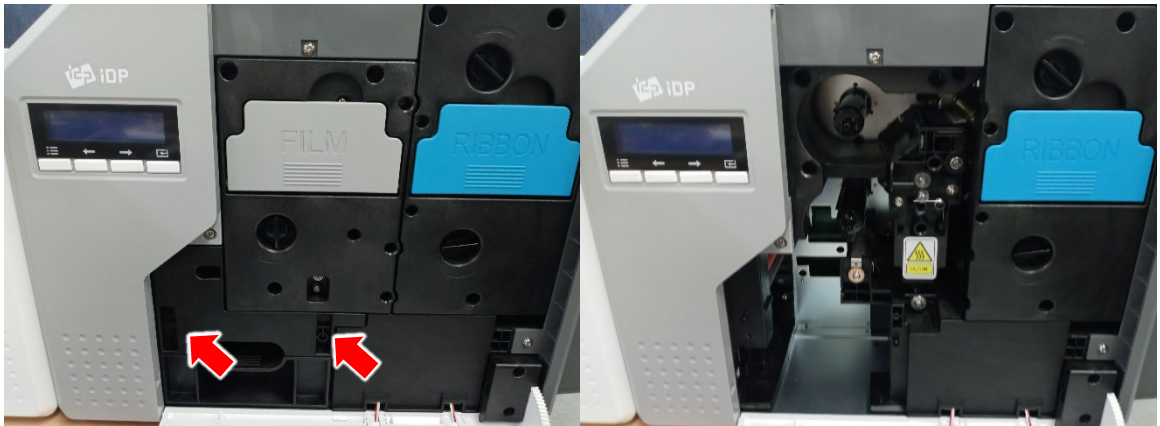
Figure 39 Take out module (IC, RF)
