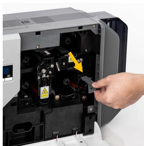
Figure 11 Take out Cleaning roller Cartridge
