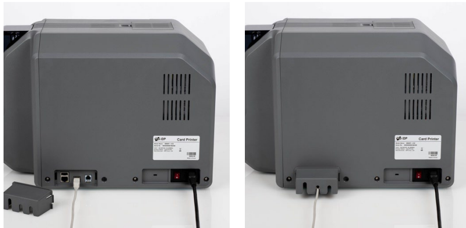
Figure 7 SMART-81 Connection of power and communication cable
